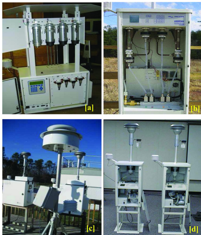
Figure 15. PM 2.5 speciation samplers (62).
