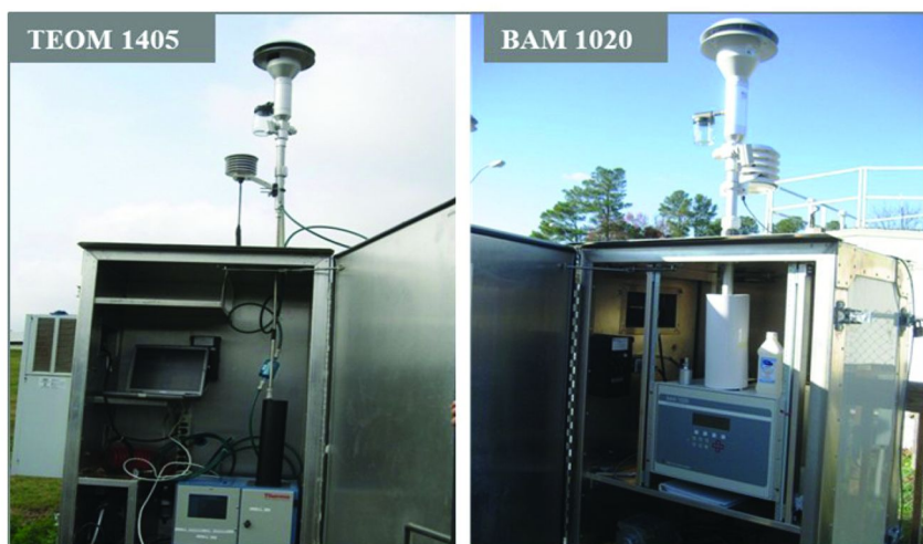
Figure 10. Automated PM monitors: FEM TEOM- PM_{10} (left) & BAM- PM_{2.5} ( PM_{10} head + VSCC) (right).
